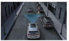
Autonomous Emergency Braking (AEB)
